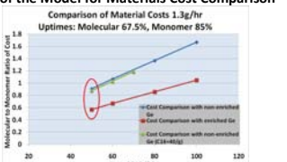
FIGURE 4. Shows is the source materials cost comparison for the molecular to the monomer tool operation as a ratio against both enriched and non-enriched Ge operation.
